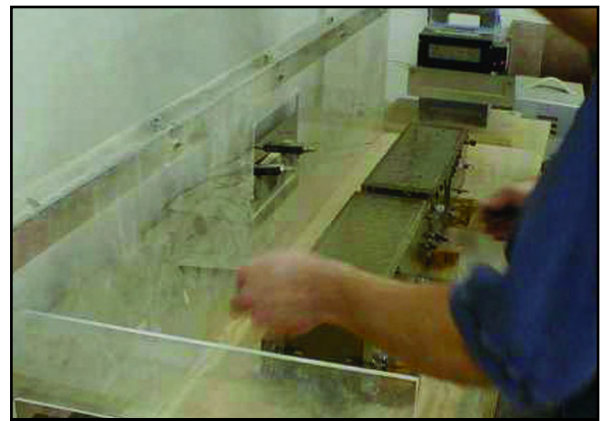
Figure 4. Placing Overlay into Chamber
